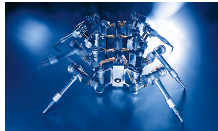
Scorpion, eight-legged walking robot for outdoor terrain designed by Prof. Dr. Frank Kirchner, head of the Robotics Innovation Center at DFKI in Bremen © Dieter Klein
